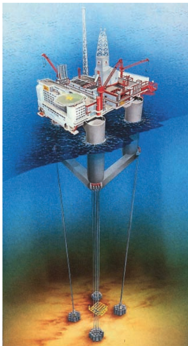
The Heidrun TLP with its steel tethers. Illustration: Statoil
