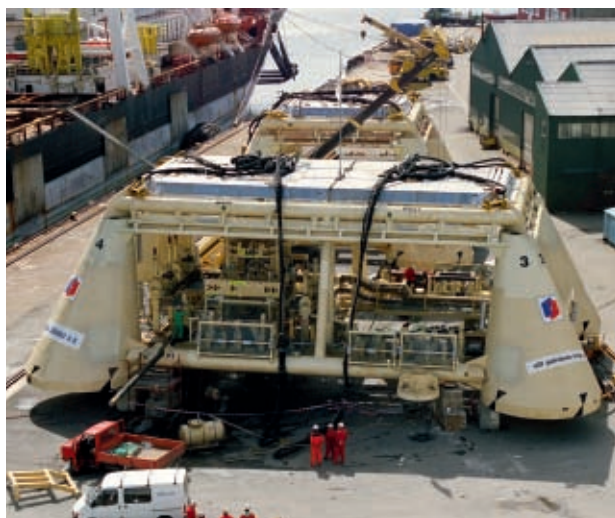
A Lille-Frigg subsea template. Photo: Elf
